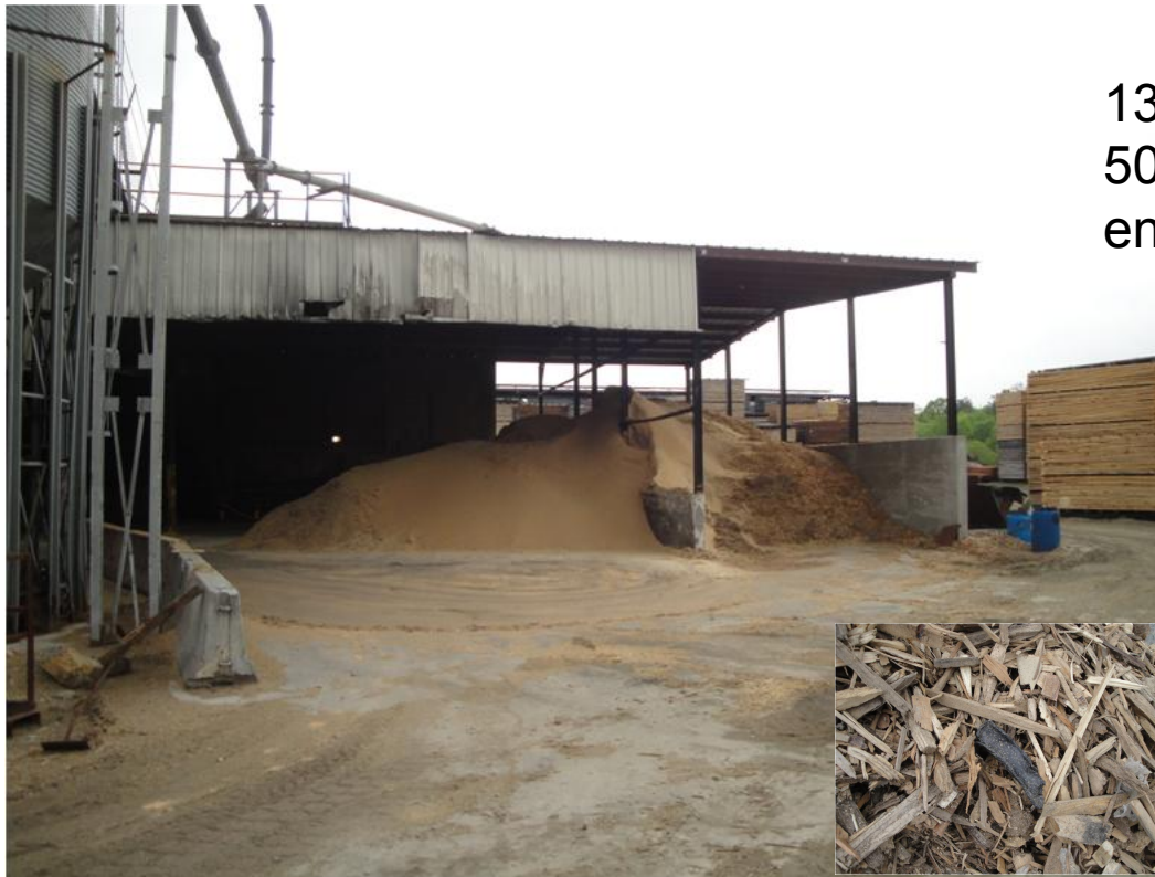
Use of sawdust as boiler fuel. VA.
