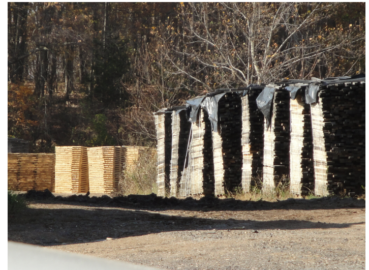
Barrel staves in the air-dry seasoning process. VA
